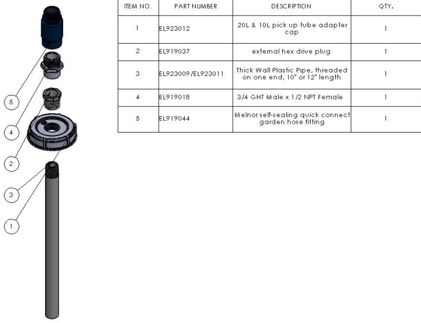
Figure 11: Pick Up Tube Adapter, Exploded View
