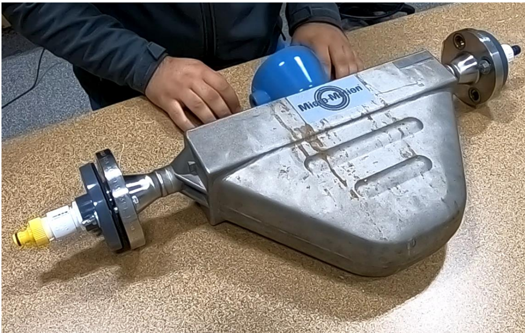
Figure 5: Flow Meter secured with appropriate flange adapters.
