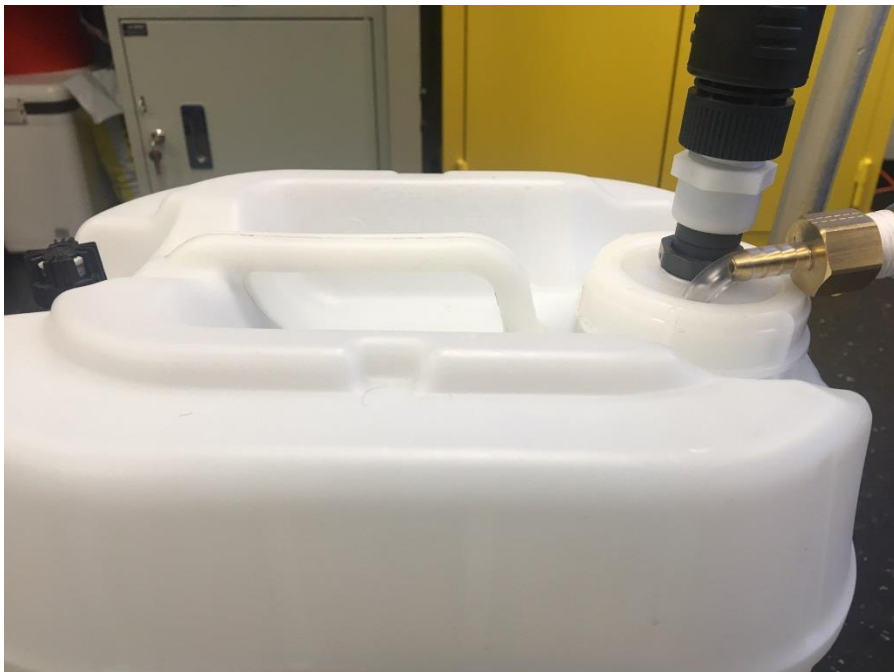
Figure 9: Adapter cap with pick up tube and tank return hose attached.
