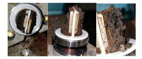
Figure 2: 2" untreated Vortex meter caked with paraffin fouling after 50-60 days of operations.
