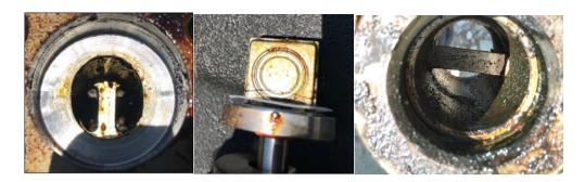
Figure 3: e9 Pro Performance treated 2" Vortex meter with minimal deposition after 80 days of operations.
