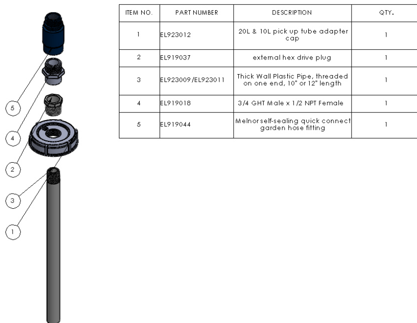
Figure 11: Pick Up Tube Adapter, Exploded View
