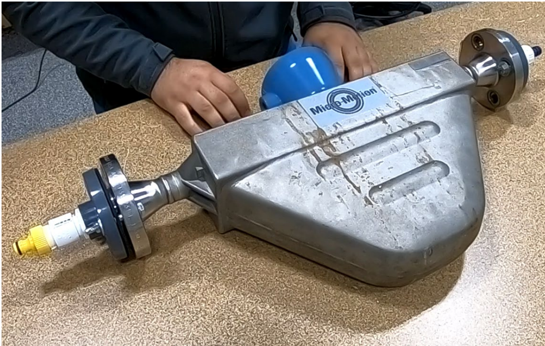
Figure 5: Flow Meter secured with appropriate flange adapters.
