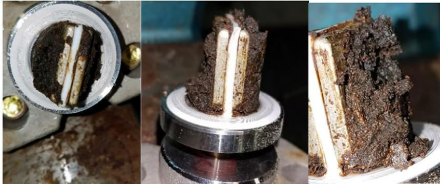
**Figure 2: 2" untreated Vortex meter caked with paraffin fouling after 50-60 days of operations.**
