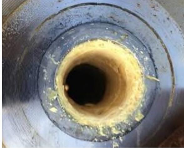
**Figure 4: Image showing paraffin deposition on the walls of the flow cavity of an untreated multiphase flow meter.**
