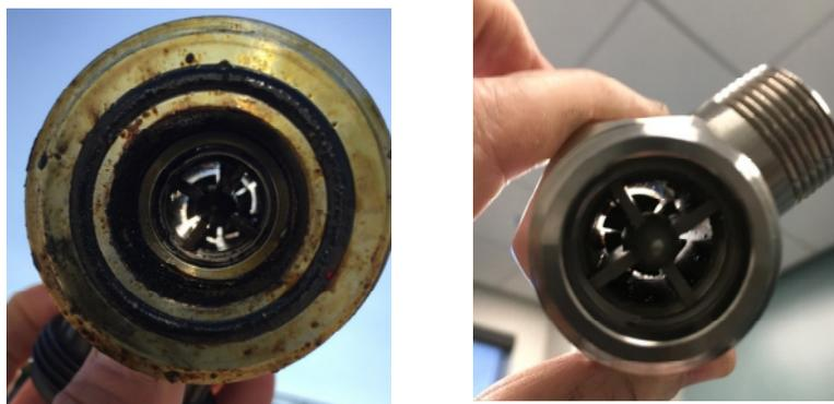
**Figure 1: 1" NPT treated Turbine meter (left) while operational in the field; (right) after proving without any cleaning process.**
